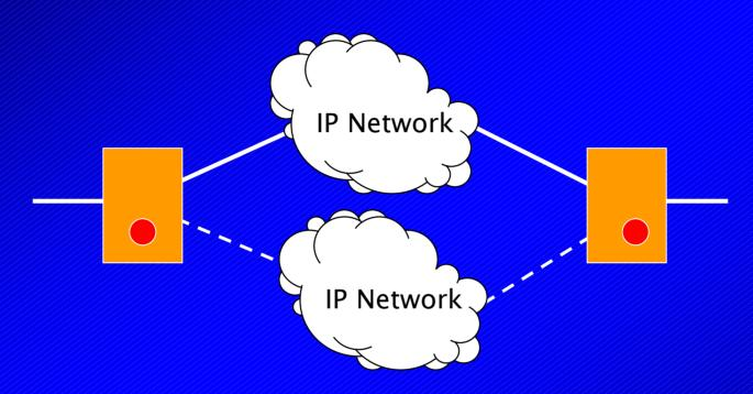
Select route based on estimate of subjective quality metric - not components Monitor live calls on active route Generate test calls on inactive route
