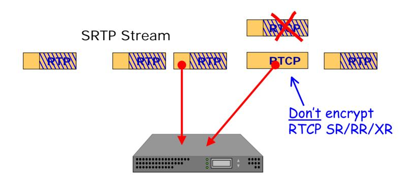
Probes, analyzers and voice quality testers <u>can</u> decode RTP headers and <u>can</u> make use of RTCP SR/RR/XR metrics
