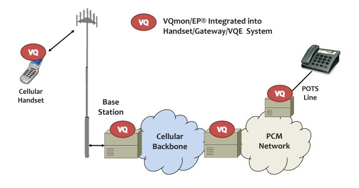
Figure 2: VQmon integration into cellular handset and network elements
